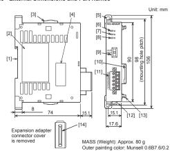
[1] DIN rail mounting groove
